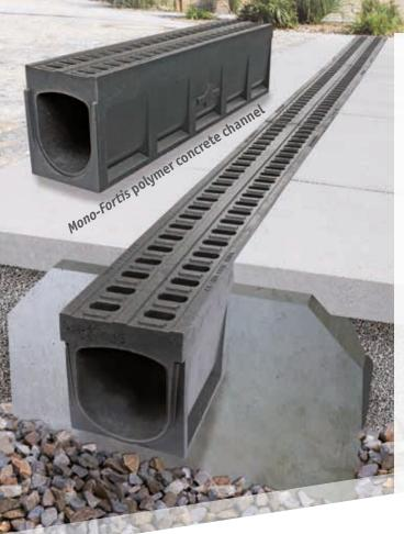
The new **Mono-Fortis** heavy-duty channel is made from polymer concrete and unites channel and grating in one. The channel's eponymous, monolithic construction ensures its stability up to load class E 600. The channels are produced in lengths of one metre, with an inlet width of 206mm (DN 150) and a height of 250mm.
