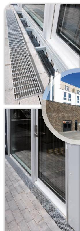
High in the sky – custom-made 470 mm high façade channels accompany the buildings on the shopping centre roof-top. The 15 mm protruding supporting base for the gratings **a** and the channel bases **b** – also installed with 15 mm of space – ensure a consistent distance from the base areas of the apartment buildings.
