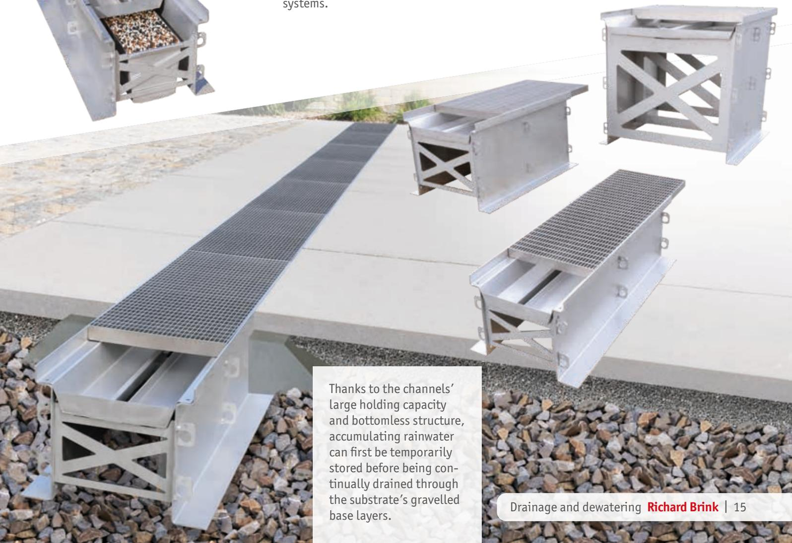
Thanks to the channels' large holding capacity and bottomless structure, accumulating rainwater can first be temporarily stored before being continually drained through the substrate's gravelled base layers.
