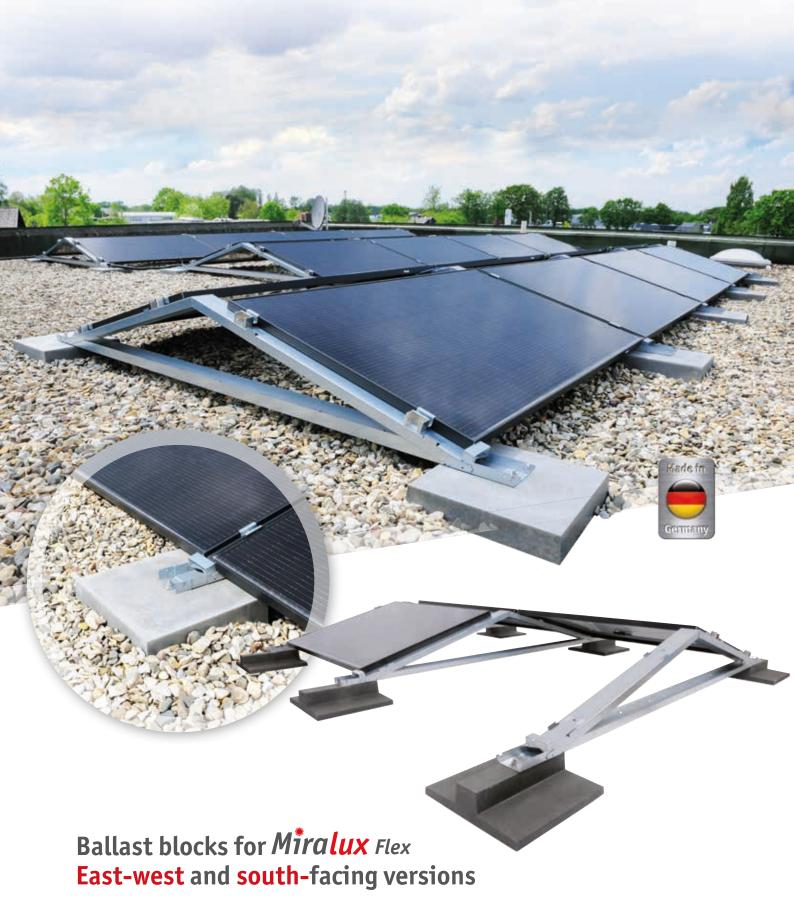
Our ballast blocks made from polymer concrete have a base area of 400 x 400mm and ensure a stable and safe installation of the solar substructures on gravel and green roofs. Besides the increased safety gained from fixing the solar substructures in
